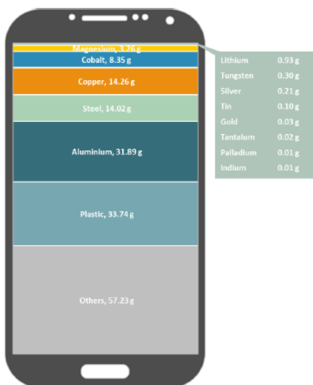
Figure 5: Estimated composition of a mobile phone (EESC, 2019)
