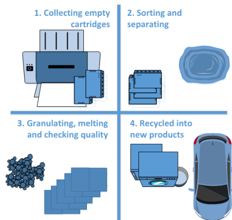
Figure 32: Recycling process for Samsung cartridges
