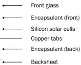
Figure 7. Cross section of a contemporary standard PV panel
