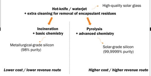
Figure 4. Recycling routes incineration and pyrolysis
