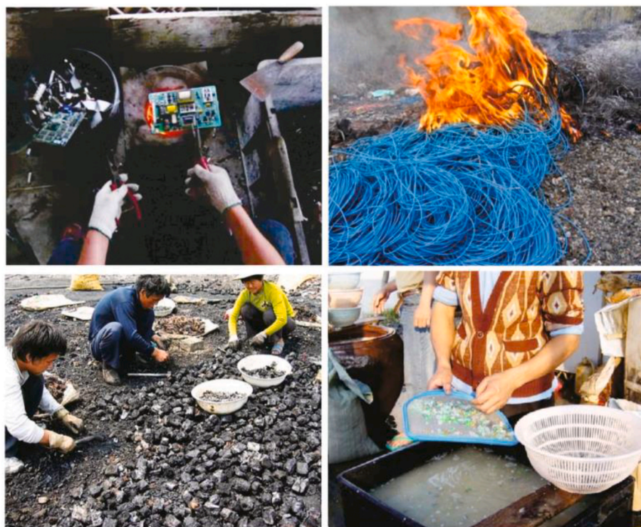
Fig. 2. Informal e-waste recycling activities, including circuit board baking (a), wire burning (b), dismantling (c), and acid leaching (d) in Guiyu, China (Source: Xu et al., 2015. Permission to publish the figure was obtained from the Licensed Content Publisher Springer Nature, License Number: 4914780066481 and License date: September 23, 2020).
