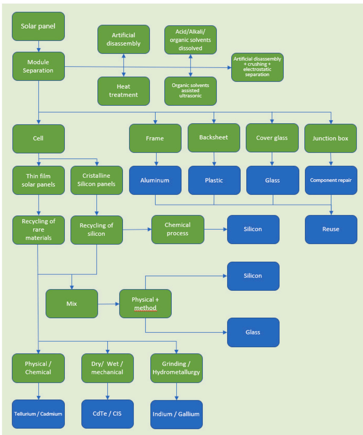
Fig. 5. Recycling techniques per module type. Source: The authors of this study, adapted from Xu et al. (2018)
