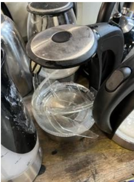
1 Gebroken waterkokers (glas) en gescheurde waterkokers (plastic).
