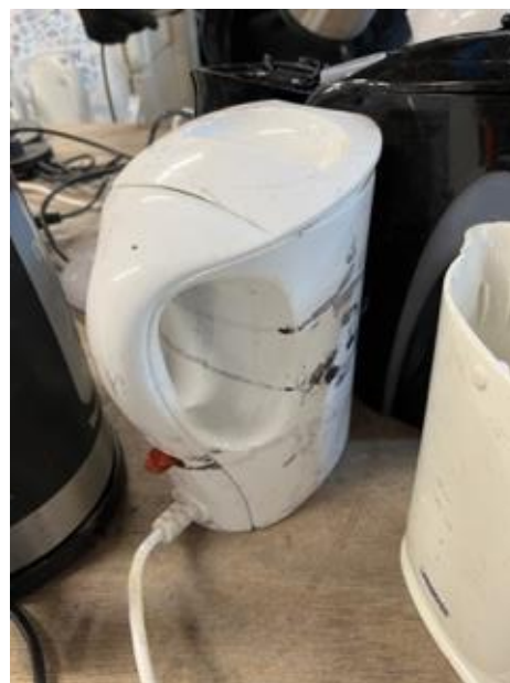
1 Gebroken waterkokers (glas) en gescheurde waterkokers (plastic).
