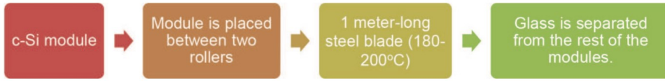
Figure 1.8.: Flowchart of the “hot knife” process used to remove glass sheet from PV modules [39].
