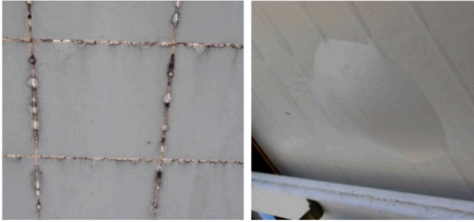
Figure 1.2.: Examples of backsheet degradation and failure: cracking (left) and delamination (right) [18].
